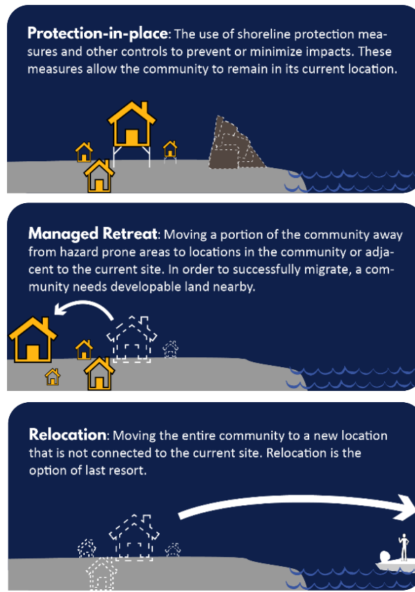
Figure 15. Common types of solutions to climate impacts to infrastructure in Alaska Native communities. Source: DeLue, M.; Alaska Climate Adaptation Science Center. ANTHC, DCRA, et al., draft report.
